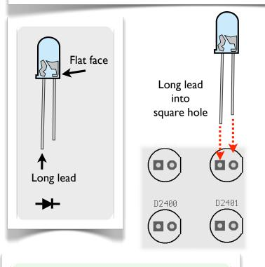
Alternative build idea: put all the LEDs on the back side of the circuit board for truly bare background. In this scheme, the long lead still goes in the square hole.
