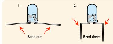
Where the grid *really* won't do, you can put LEDs *between* grid locations. Which ever way you do it, the side of each LED with long lead *still* goes to square hole. Side with flat *still* goes to round hole.
